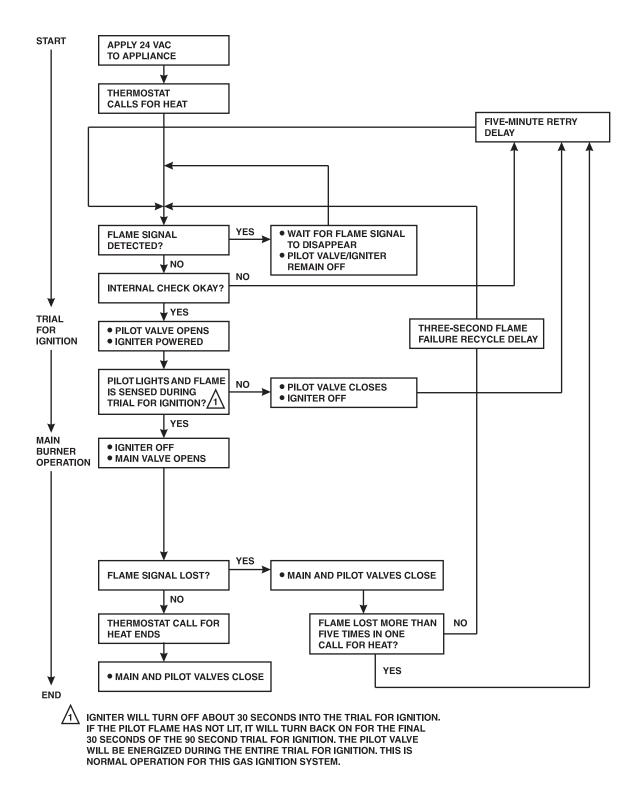
Figure 6.4: Intermittent Ignition System Operating Sequence
